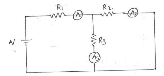
**5. PROCEDURE:** Three rheostats  $R_1$ ,  $R_2$  and  $R_3$  and ammeters  $A_1$ ,  $A_2$  and  $A_3$  are connected to 24 V battery or regulated power supply as shown in figure. The three rheostats are set their maximum values, supply is switched on and the reading of the ammeter  $A_1$ ,  $A_2$  and  $A_3$  are noted. The process may be repeated by varying either of rheostats  $R_1$ ,  $R_2$  and  $R_3$ .
