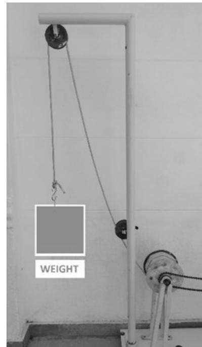
Fig 5: Rope, drum and load arrangement
