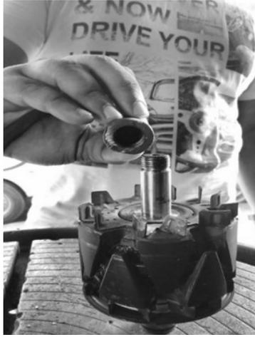
Fig 8: Field of an alternator
