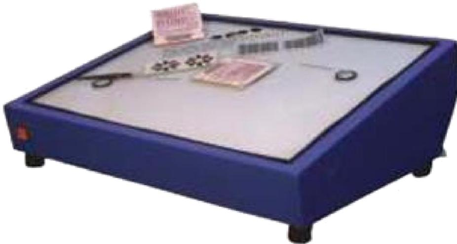
The PCB Drafting Kit includes Various tapes, pad and other material for making PCB Artworks.
