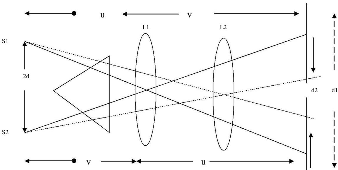
Fig. 3 Determination of distance between two sources
