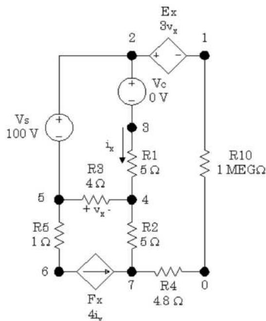
In this example, we want the Thévenin equivalent circuit from nodes 1 to 0. The 1 Megohm resistor is placed in the circuit because PSpice requires at least two connections to each node. This resistor is large enough that it will not have an effect on the calculations. Note the use of voltage source Vc which has the purpose of monitoring the control current,  $i_x$ , used for the current-controlled dependent current source, Fx. The input lines in the \*.CIR file are shown below.
