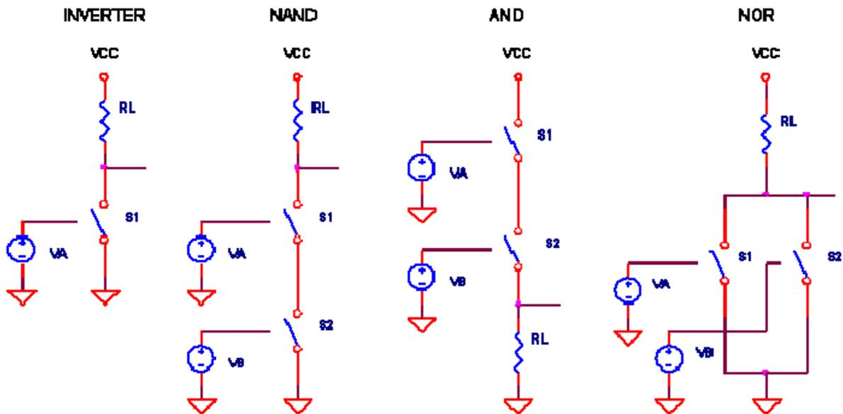
You're simulating a circuit, it requires several digital gates, but you don't have a mixed-mode simulator. What to do? One solution involves creating simplified versions of the logic functions.
