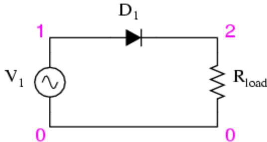
In half wave rectification, either the positive or negative half of the AC wave is passed, while the other half is blocked. Because only one half of the input waveform reaches the output, it is very inefficient if used for power transfer. Half-wave rectification can be achieved with a single diode in a one-phase supply, or with three diodes in a three-phase supply. Half wave rectifiers yield a unidirectional but pulsating direct current.
