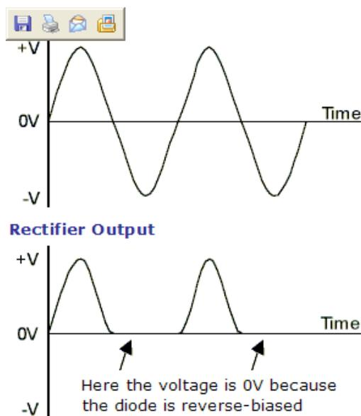
Figure : Half-wave rectification
