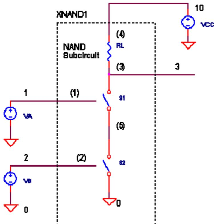
S1 and S2 are defined by  $R_{ON} = 10 \Omega$  and  $R_{OFF} = 1 M\Omega$ . Compared to the other resistances in the circuit, these should look like an ideal switches. More on the SPICE switch below.
