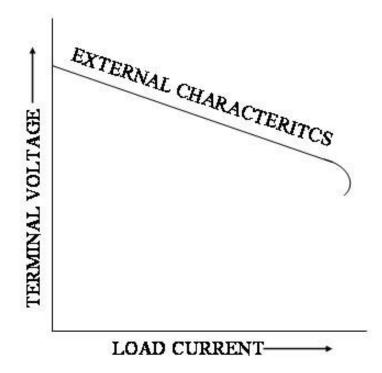
External characteristics of a DC Shunt Generator.
