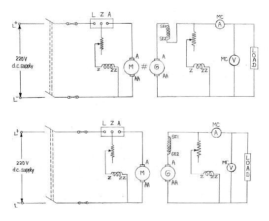
Fig1 : Load test on DC generator.
