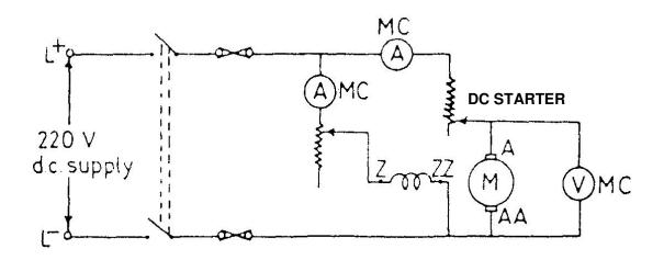
Fig 'A' (i) : Schematic Diagram for Swinburne's test on DC Motor.
