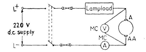
Fig 'A' (ii) : Schematic diagram for Measurement of armature resistance
