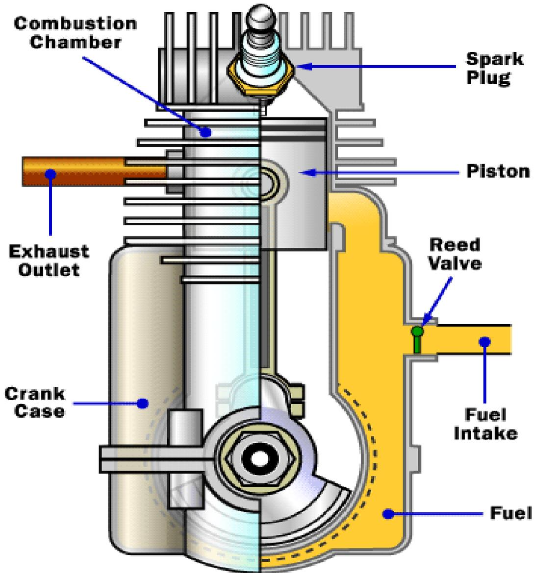
**The basic components of a two-stroke engine**
