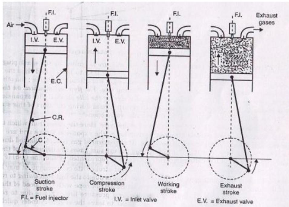
**Fig. Four-stroke Diesel cycle engine**
