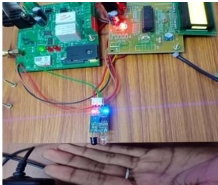
Fig.11IR Sensor detects the object
