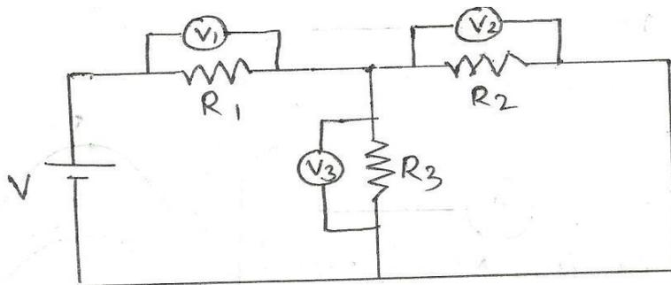
5. PROCEDURE: Two rheostats  $R_1$ ,  $R_2$ ,  $R_3$  and three voltmeters  $V_1$ ,  $V_2$  and  $V_3$  are connected to 24V battery or regulated power supply as shown in figure. Three rheostats are set their maximum values, supply is switched on and the reading of the voltmeters  $V_1$ ,  $V_2$  and  $V_3$  are noted. The process may be repeated by varying either of rheostats  $R_1$ ,  $R_2$  or  $R_3$ .
