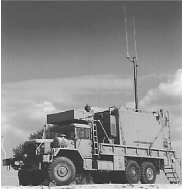
Figure 13.7 Hermes UAV GCS vehicle
