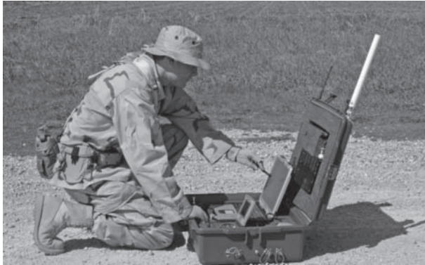
Figure 13.2 Desert Hawk GCS. (Reproduced by permission of Lockheed Martin Corp)
