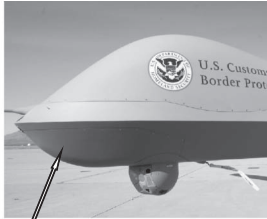
LYNX I installed is installed in Predator Nose
