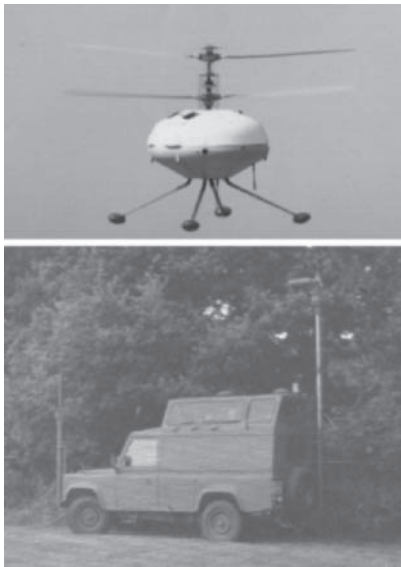
Figure 4.19 ML Aviation Sprite close-range VTOL UAV
