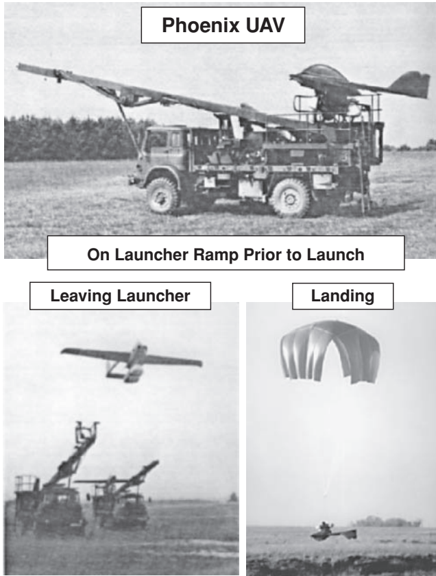
Figure 12.4 Phoenix – launch to landing
