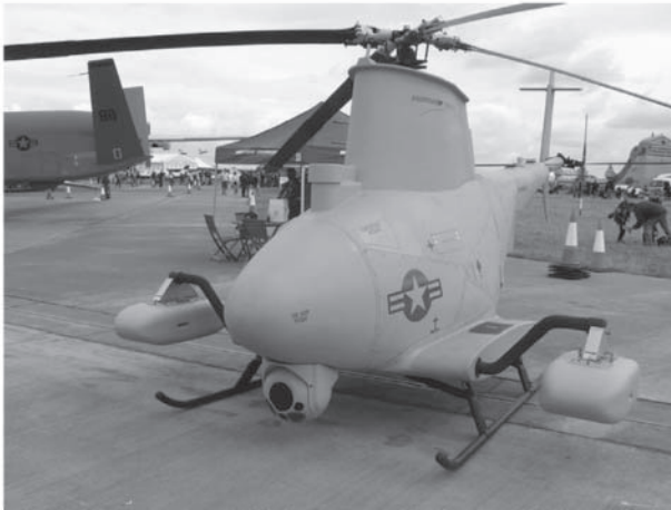
Northrop Grumman RQ8 "Fire Scout" Armed with rockets in side-mounted pods
