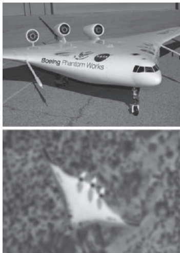
Figure 4.29 Blended wing-body model
