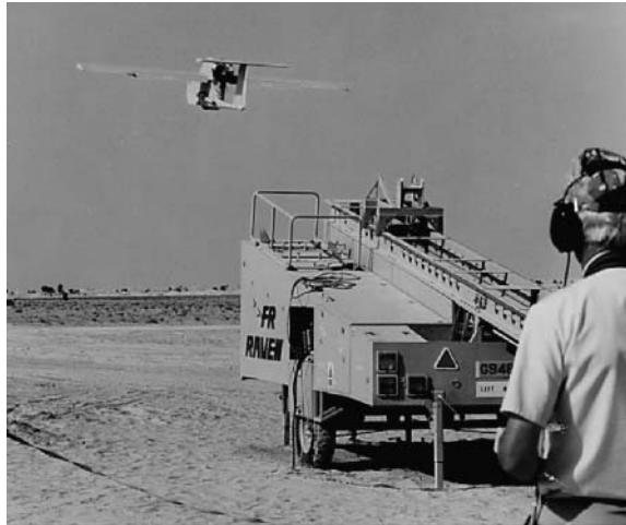
Figure 15.3 Raven UAV launch from trailer
