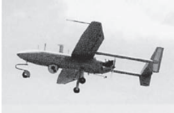
Figure 4.11 Medium-range UAV: Hunter and Seeker (Reproduced by permission of Denel Aerospace). Source: Israeli Aircraft Industries
