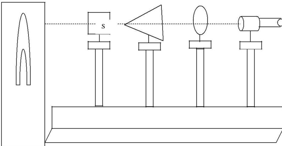
Fig. 1 Experimental arrangement of Biprism
