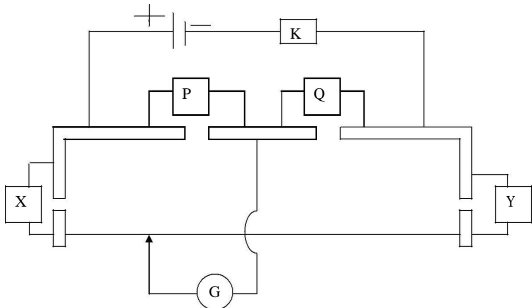
**Method:** **Low resistance by calibrating the bridge – wire:** Let  $x$  be the unknown resistance and  $d_1, d_2$  shifts obtained with resistance  $Y_1$  and  $Y_2$  the know resistance box then
