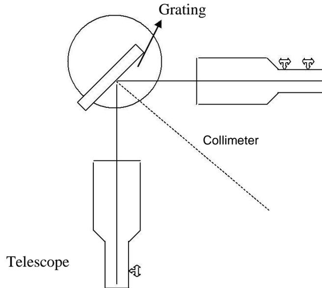
**Adjustment of grating for normal incidence (step 1-3)**
