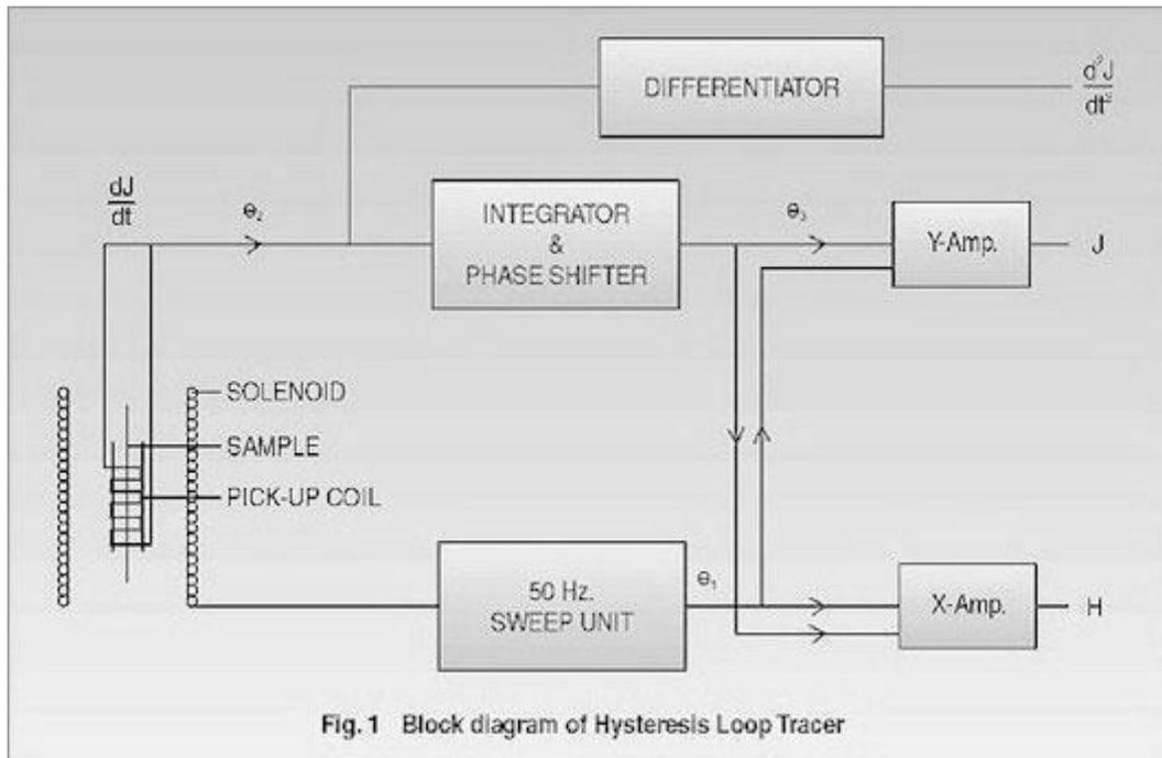
2. Now adjust the knob of magnetic field in the hysteresis loop tracer to minimum value say 30Gauss. Note down the loop width in mm, Tip to tip height (mV) as shown in fig.
