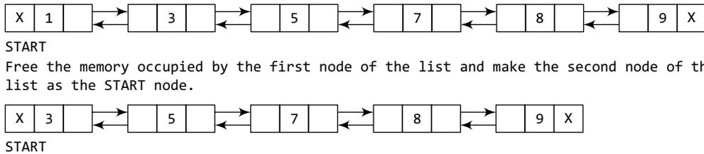
**Figure 6.47** Deleting the first node from a doubly linked list
