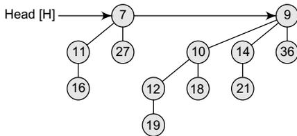
Figure 12.13 Binomial heap
