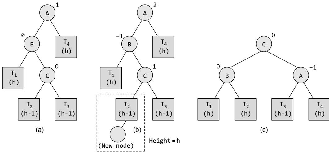
Figure 10.44 LR rotation in an AVL tree
