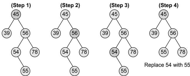
**Figure 10.12** Deleting node 54 from the given binary search tree
