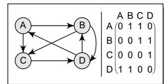
Figure 13.39 Graph  $G$  and its path matrix  $P$
