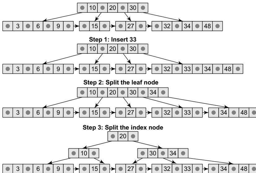
**Figure 11.11** Inserting node 33 in the given B+ Tree
