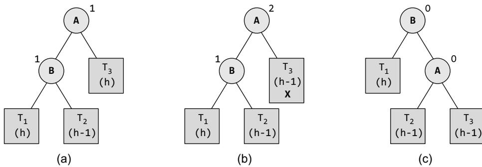
Figure 10.50 R1 rotation in an AVL tree
