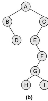
**Example 9.6** In Figs (a) and (b), find the sequence of nodes that will be visited using pre-order traversal algorithm.
