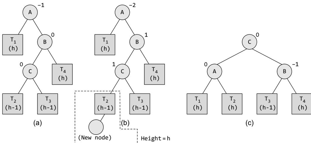
Figure 10.46 RL rotation in an AVL tree
