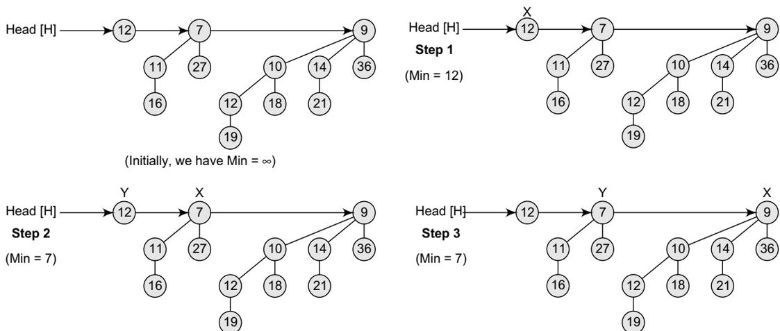
**Figure 12.16** Binomial heap
