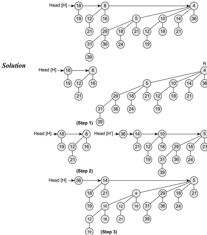
Figure 12.22 Binomial heap
