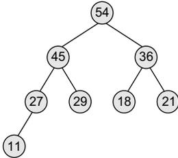
Figure 12.8 Binary heap
