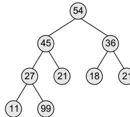
**Figure 12.3** Binary heap after insertion of 99
