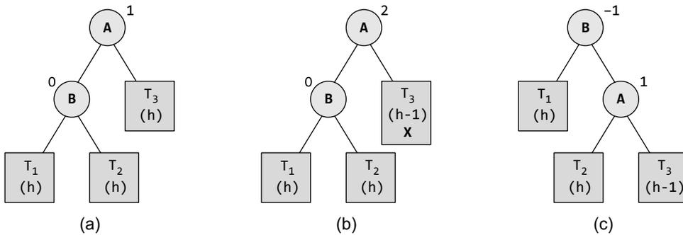
Figure 10.48 R0 rotation in an AVL tree
