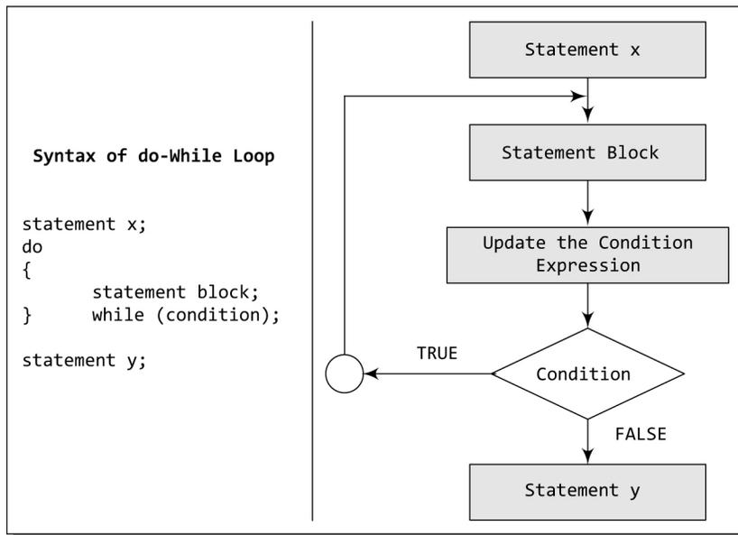
**Figure 1.7** Do-while construct
