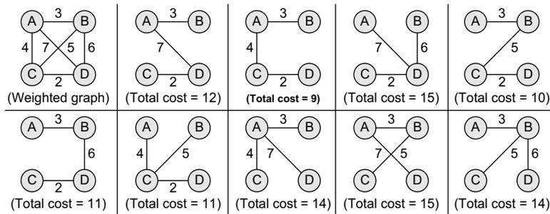
Figure 13.29 Weighted graph and its spanning trees
