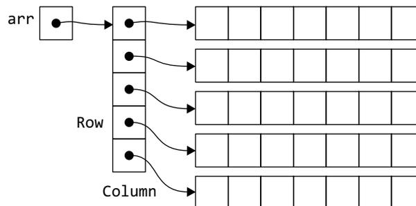
**Figure A2** Memory allocation of two-dimensional array
