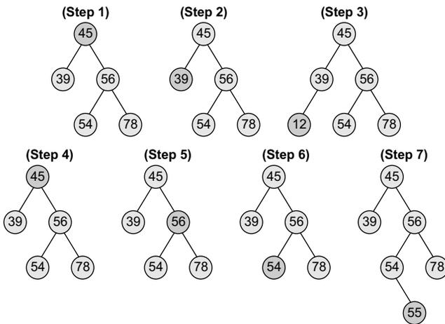
**Figure 10.10** Inserting nodes with values 12 and 55 in the given binary search tree
