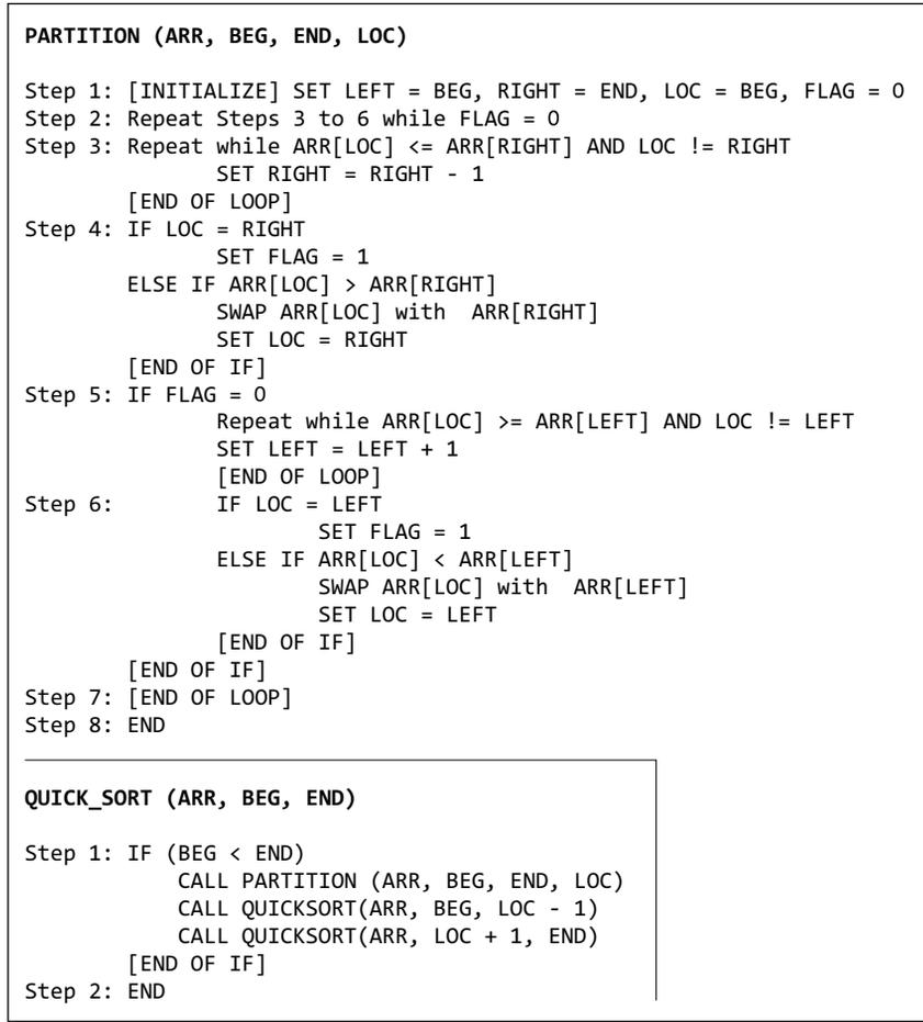
**Figure 14.10** Algorithm for quick sort
