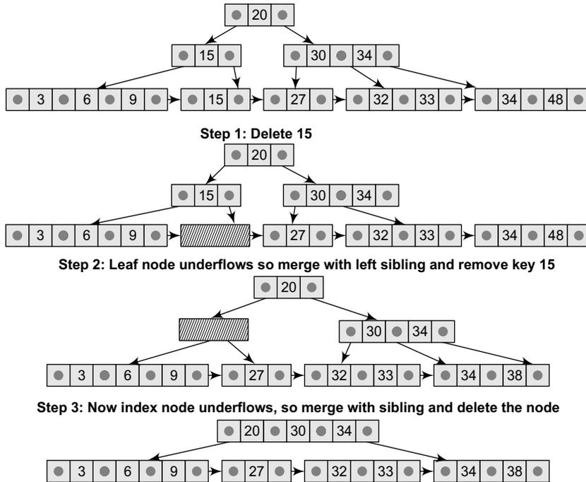
**Figure 11.13** Deleting node 15 from the given B+ Tree
