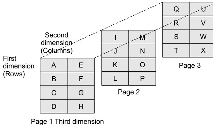
**Figure 3.33** Three-dimensional array
