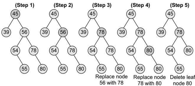
**Figure 10.14** Deleting node 56 from the given binary search tree
