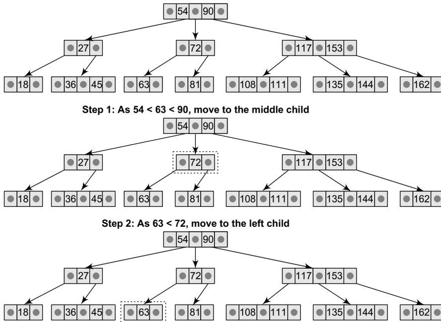
**Figure 11.15** Searching for element 63 in the 2-3 tree of Fig. 11.14
