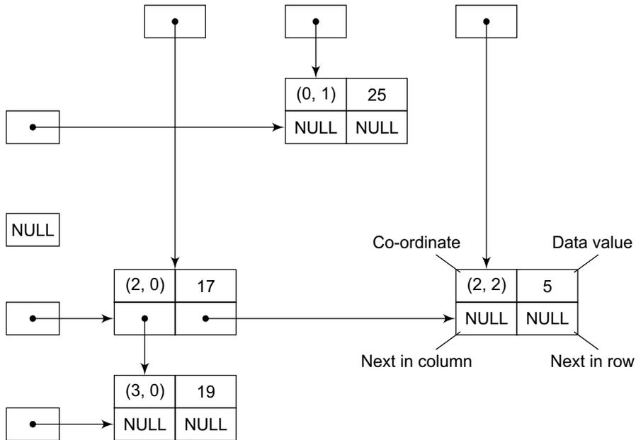
Figure 6.73 Multi-linked representation of sparse matrix shown in Fig. 6.72
