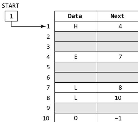
**Figure 6.2** *START* pointing to the first element of the linked list in the memory
