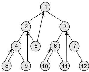
Figure 10.30 (b) Binary tree with one-way threading
