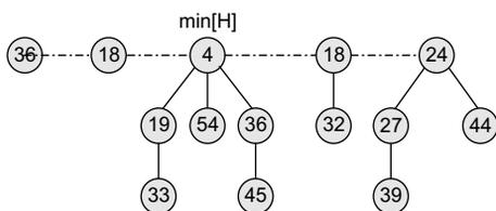
Figure 12.26 Fibonacci heap
