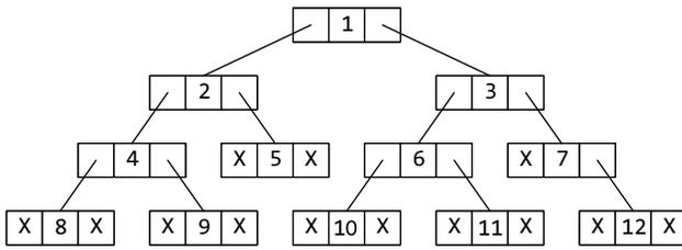
Figure 10.28 Linked representation of a binary tree
