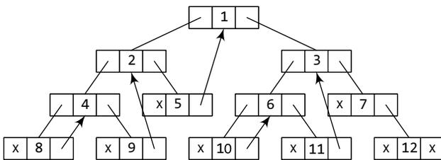
Figure 10.30 (a) Linked representation of the binary tree with one-way threading
