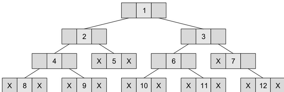
**Figure 9.9** Linked representation of a binary tree
