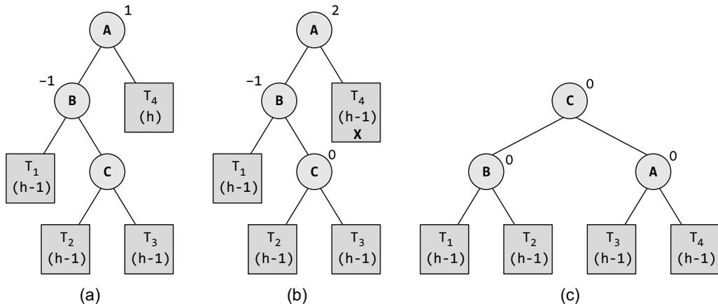
Figure 10.52 R1 Rotation in an AVL tree
