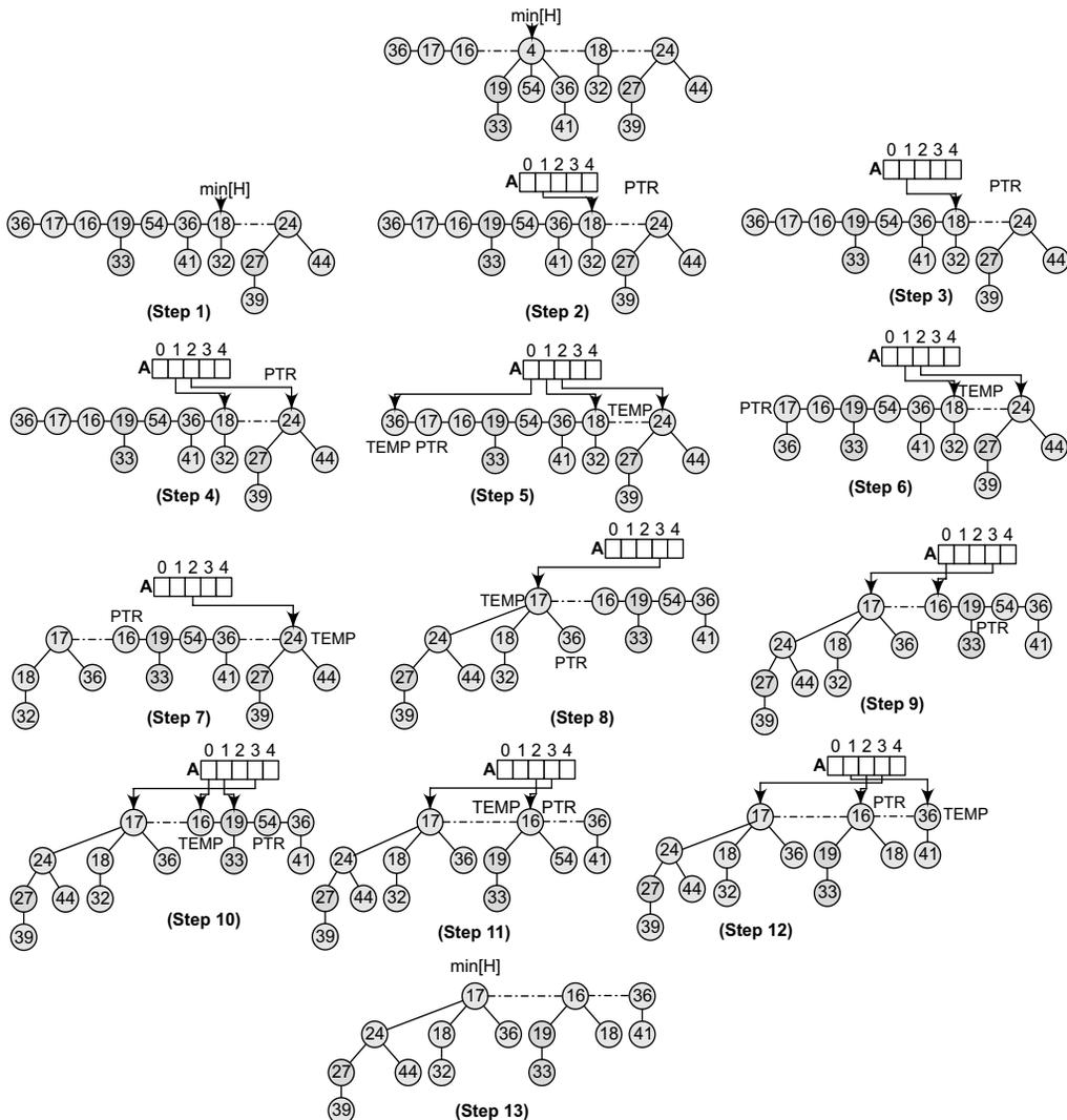
**Figure 12.34** Fibonacci heap
