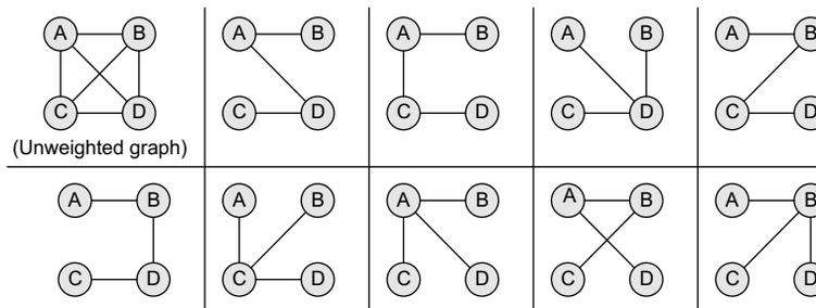
**Figure 13.28** Unweighted graph and its spanning trees
