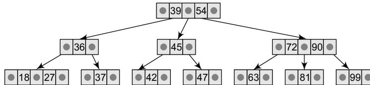
Figure 11.16(i) Inserting values in the given 2-3 Tree
