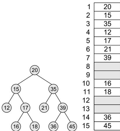
**Figure 9.12** Binary tree and its sequential representation
