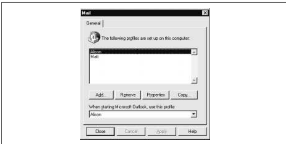
Figure 10-2. Add a profile to Outlook 98 by using the Mail or Internet Accounts window, accessed from the Control Panel
