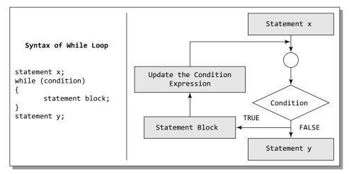
Figure 1.6 While loop construct
