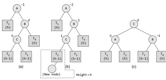
Figure 10.46 RL rotation in an AVL tree
