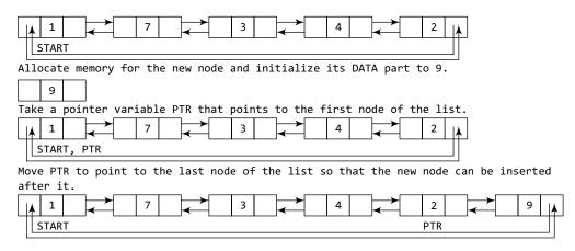
Figure 6.59 Inserting a new node at the end of a circular doubly linked list
