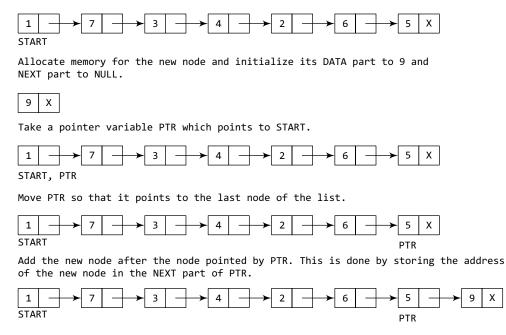
Figure 6.14 Inserting an element at the end of a linked list
