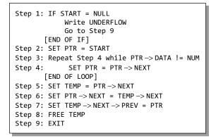
Figure 6.52 Algorithm to delete a node after a given node
