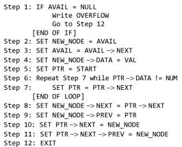
Figure 6.42 Algorithm to insert a new node at the end
