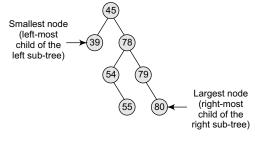
Figure 10.26 Algorithm to find the largest node in a binary search tree
