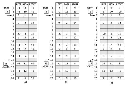
Figure 10.32 Memory representation of binary trees: (a) without threading, (b) with one-way, and (c) two-way threading
