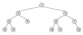
Figure 10.29 (a) Binary tree without threading
