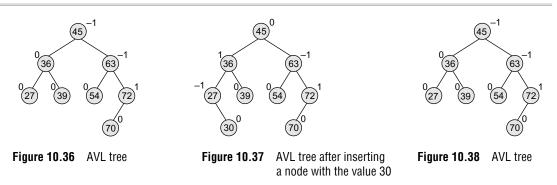
Let us take another example to see how insertion can disturb the balance factors of the nodes and how rotations are done to restore the AVL property of a tree. Look at the tree given in Fig. 10.38.
