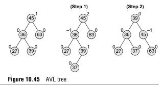
Tree (a) is an AVL tree. In tree (b), a new node is inserted in the right sub-tree of the left sub-tree of the critical node A (node A is the critical node because it is the closest ancestor whose balance factor is not -1, 0 or 1), so we apply LR rotation as shown in tree (c). Note that the new node has now become a part of tree T<sub>2</sub>.
