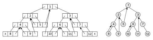
Figure 10.31 (a) Linked representation of the binary tree with threading, (b) binary tree with two-way threading
