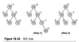
Tree (a) is an AVL tree. In tree (b), a new node is inserted in the right sub-tree of the right sub-tree of the critical node A (node A is the critical node because it is the closest ancestor whose balance factor is not -1, 0, or 1), so we apply RR rotation as shown in tree (c). Note that the new node has now become a part of tree  $T_3$ .
