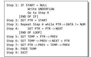
Figure 6.54 Algorithm to delete a node before a given node
