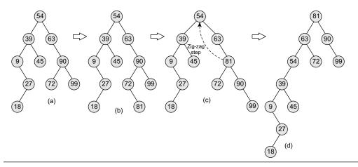
**Note** To get the final splay tree, first apply zig-zag step on 81. Then apply zig-zag step to make 81 the root node.
