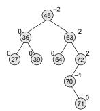
Figure 10.39 AVL tree after inserting a node with the value 71
