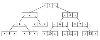
Figure 10.29 (b) Linked representation of the binary tree (without threading)
