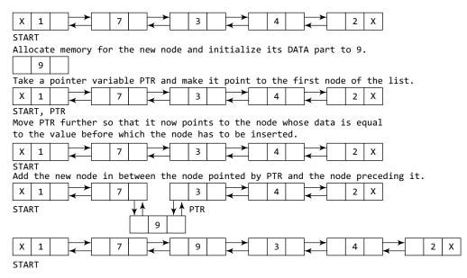
Figure 6.46 Inserting a new node before a given node in a doubly linked list
