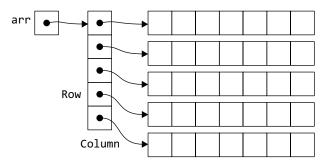
Figure A2 Memory allocation of two-dimensional array
