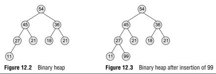
The first step says that insert the element in the heap so that the heap is a complete binary tree. So, insert the new value as the right child of node 27 in the heap. This is illustrated in Fig. 12.3.
