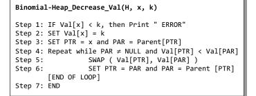
Figure 12.23 Algorithm to decrease the value of a node x in a binomial heap H
