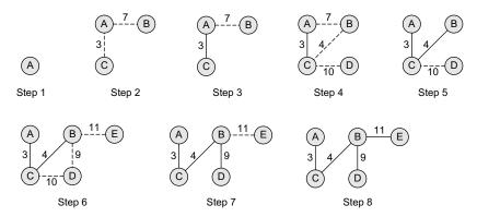
**Example 13.8** Construct a minimum spanning tree of the graph given in Fig. 13.32. Start the Prim's algorithm from vertex D.
