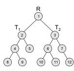
In Fig. 2.7, node 2 is the left child and node 3 is the right child of the root node 1. Note that the left sub-tree of the root node consists of the nodes 2, 4, 5, 8, and 9. Similarly, the right sub-tree of the root node consists of the nodes 3, 6, 7, 10, 11, and 12.
