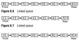
Figure 8.8 Linked queue after inserting a new node
