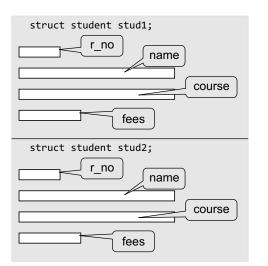
Figure 5.1 Memory allocation for a structure variable
