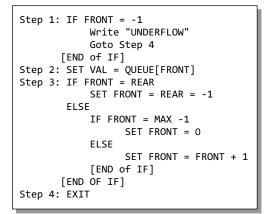
Figure 8.23 Algorithm to delete an element from a circular queue
