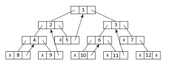
**Figure 10.30** (a) Linked representation of the binary tree with one-way threading
