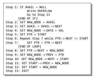
Figure 6.58 Algorithm to insert a new node at the beginning
