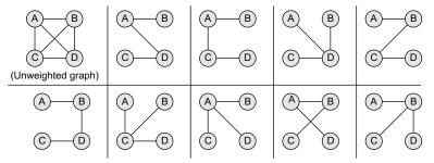
Figure 13.28 Unweighted graph and its spanning trees
