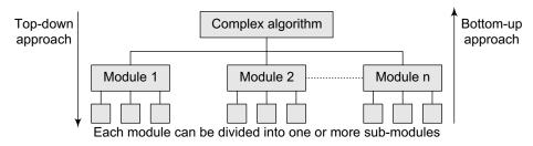
Figure 2.9 Different approaches of designing an algorithm
