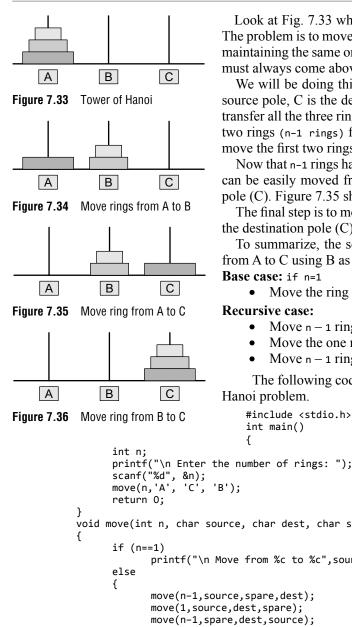
Look at Fig. 7.33 which shows three rings mounted on pole A. The problem is to move all these rings from pole A to pole C while maintaining the same order. The main issue is that the smaller disk must always come above the larger disk.
