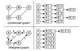
Figure 13.18 Adjacency list for an undirected graph and a weighted graph
