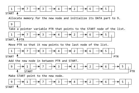
Figure 6.29 Inserting a new node at the beginning of a circular linked list
