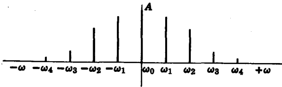
FIG. 1.4a. Discrete amplitude spectrum.
