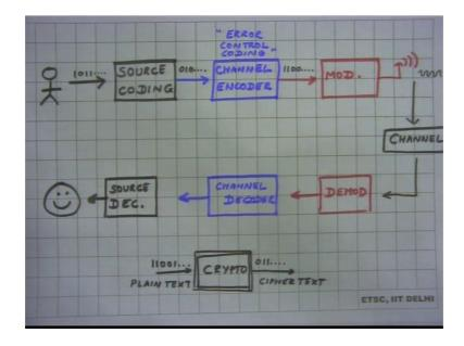
So, let us have a quick look at our communication system earlier. So, we had a source of information if you see. And then, the first block that we encountered was the source coder. The aim was the source coder was to remove the redundancy from the incoming
