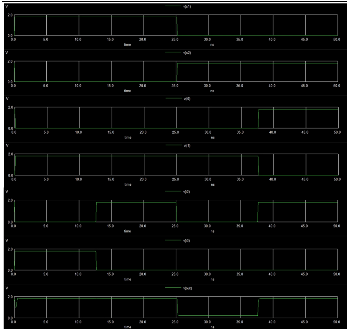
Figure:7.5 Output waveform of 4:1 multiplexer using CMOS logic
