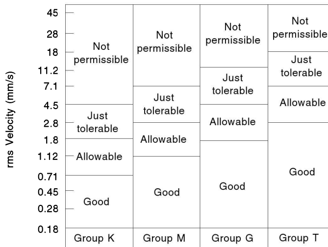
Fig. 16.12 Permissible rms levels (from VDI 2056 (1964), Courtesy: VDI Verlag GMBH, Dusseldorf)
