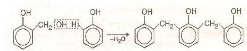
Step3: It polymerizes at high temperature into a three dimensional cross-linked polymer.
