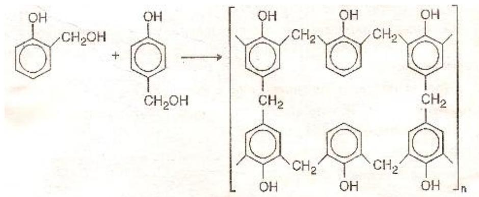
**PROCEDURE FOR PREPATION OF BAKELITE:** Take 5ml of glacial acetic acid and 2.5ml of 40% formaldehyde solution in a beaker. To this add 2ml of phenol. Add 5ml of Conc. HCl acid to the reaction mixture drop wise with continuous stirring till pink colour mass appears. Residue obtained is washed with water several times till it is free from acid. Filter and dry the product and note its weight.
