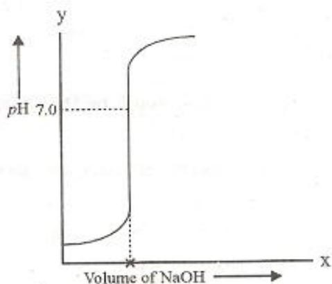
Plot between pH and volume of NaOH
