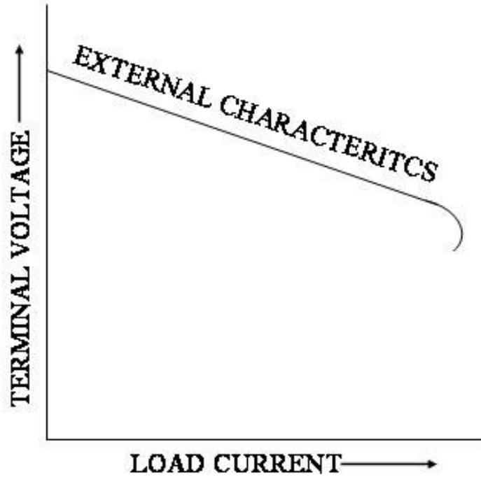
*External characteristics of a DC Shunt Generator.*
