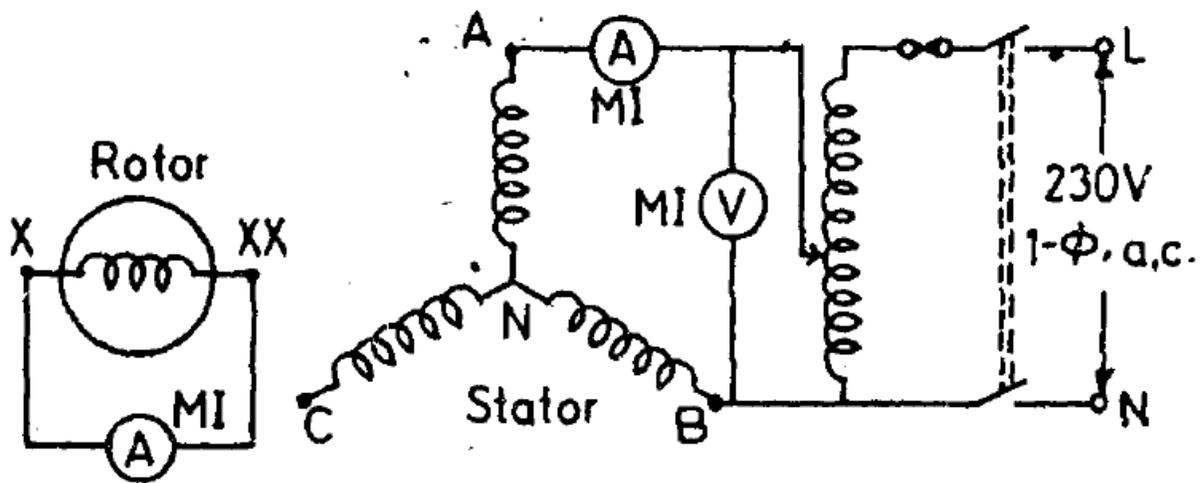
1. Let the applied voltage across the terminals A,B of the stator winding with terminal C kept isolated be E volts and the current flowing through the winding in current be I amperes. The ratio of voltage across each phase to current is a reactance which can be represented by a quantity A' i.e.
